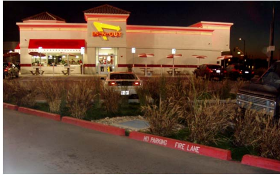
Rain garden in parking lot island.
